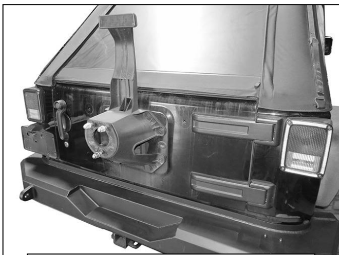
(Fig 1) Unplug and remove 3rd brake light assembly from factory spare tire mount
