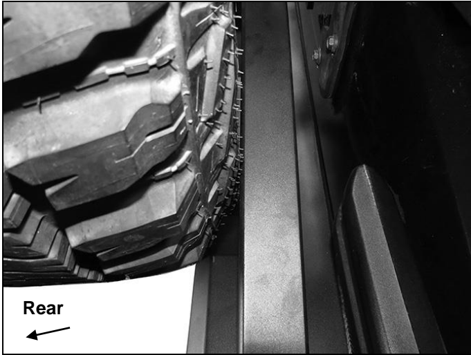
(Fig 19) Adjust Brackets so that tire is in contact with Arm. Temporarily remove spare tire
