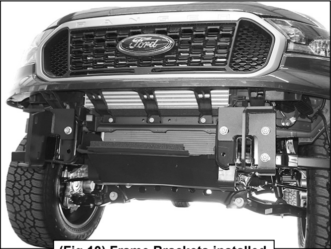
(Fig 10) Frame Brackets installed
