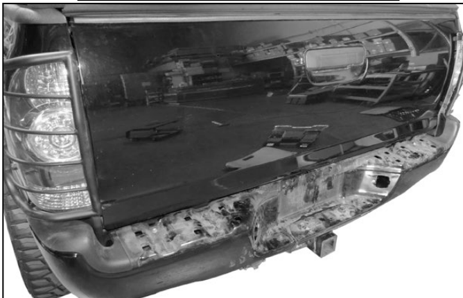
(Fig 3) Models with receiver hitch only, remove plastic cover from top of bumper to access hex bolts attaching bumper to top of receiver hitch
