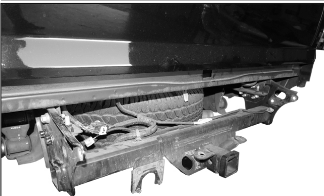
(Fig 3) Models with receiver hitch only, remove plastic cover from top of bumper to access hex bolts attaching bumper to top of receiver hitch
