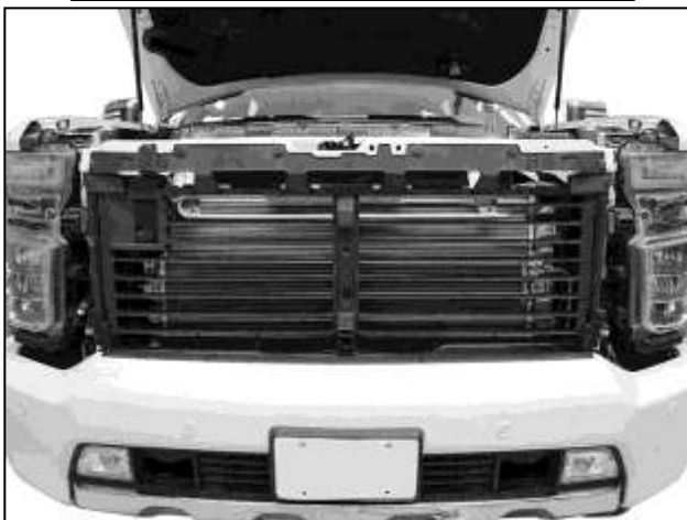
(Fig 7) Grille and fascia removed
