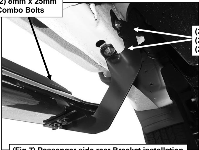
(Fig 7) Passenger side rear Bracket installation
