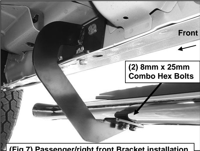
(Fig 7) Passenger/right front Bracket installation
