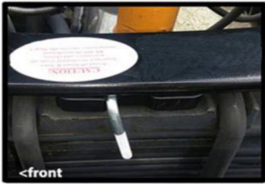
Place PSP-11 on top of spring plate flat side up with groove toward the front
