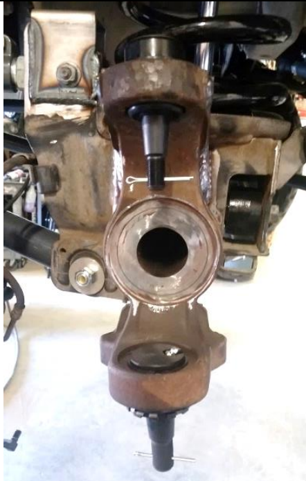
Figure 13. Cotter Pins Aligned Front to Back
