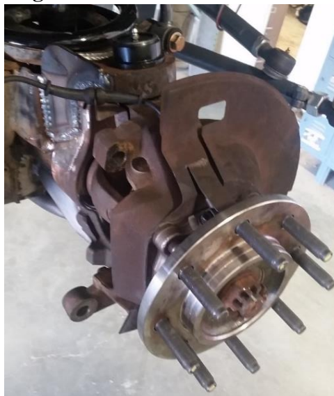
Figure 16. Backing Plates, Hubs and ABS Lines Re-Installed
