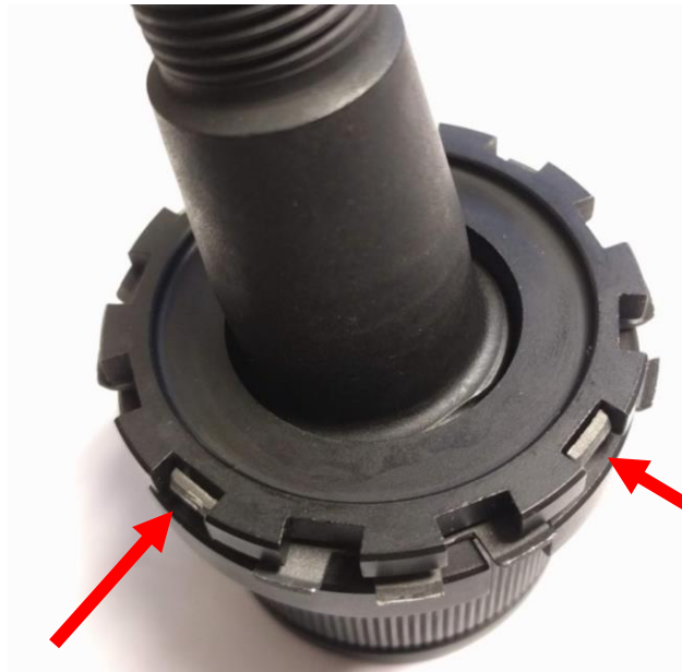
Figure 15. Tabs Bent Into the Cap
