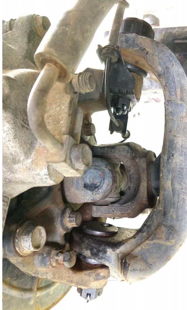
Figure 16. Finished Ball Joint Installation
