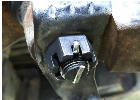
Figure 14. Cotter Pin Installed
