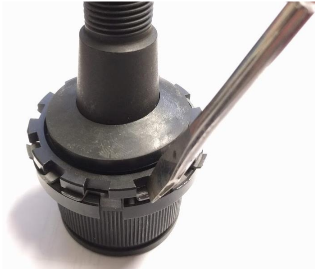
Figure 18. Bending Locking Tabs Back
