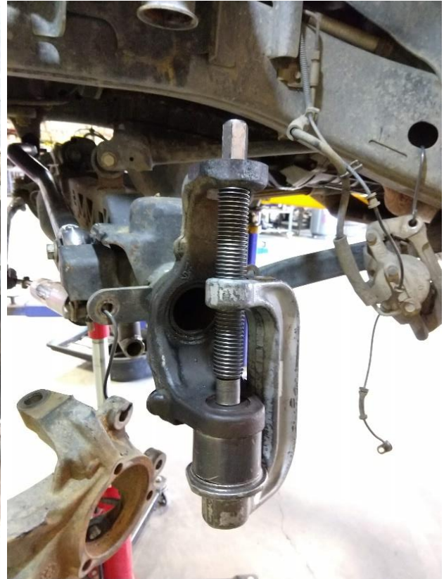
Figure 9. Pressing Out Lower Ball Joint
