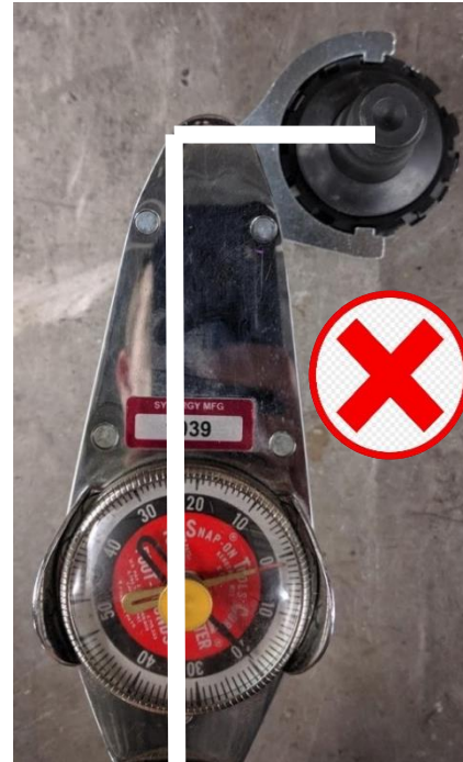
Figure 20. Incorrect Wrench Orientation
