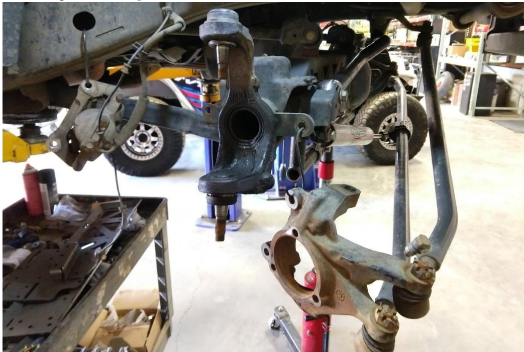
Figure 7. Knuckle Removed, Hanging from Axle Housing
