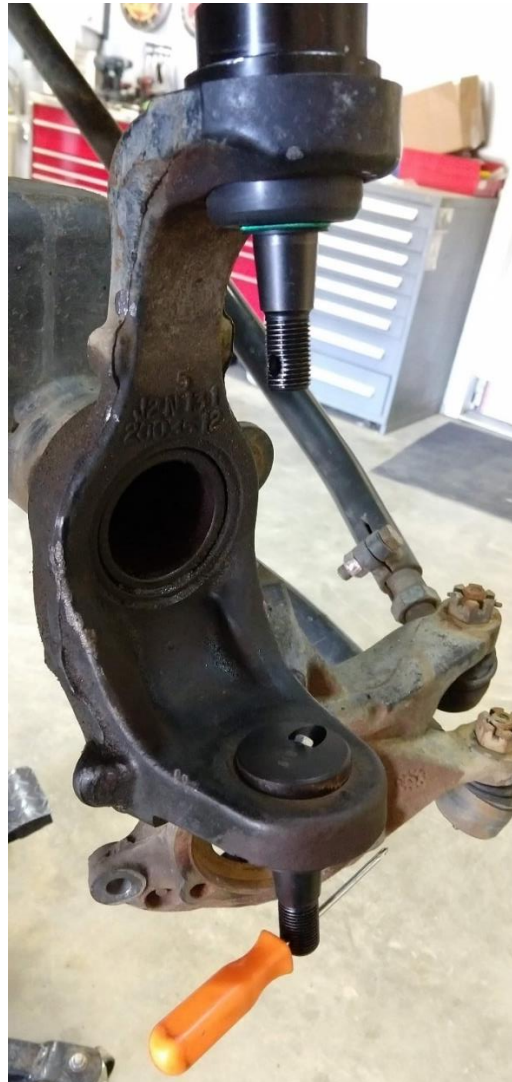
Figure 13. Cotter Pins Aligned Front to Back
