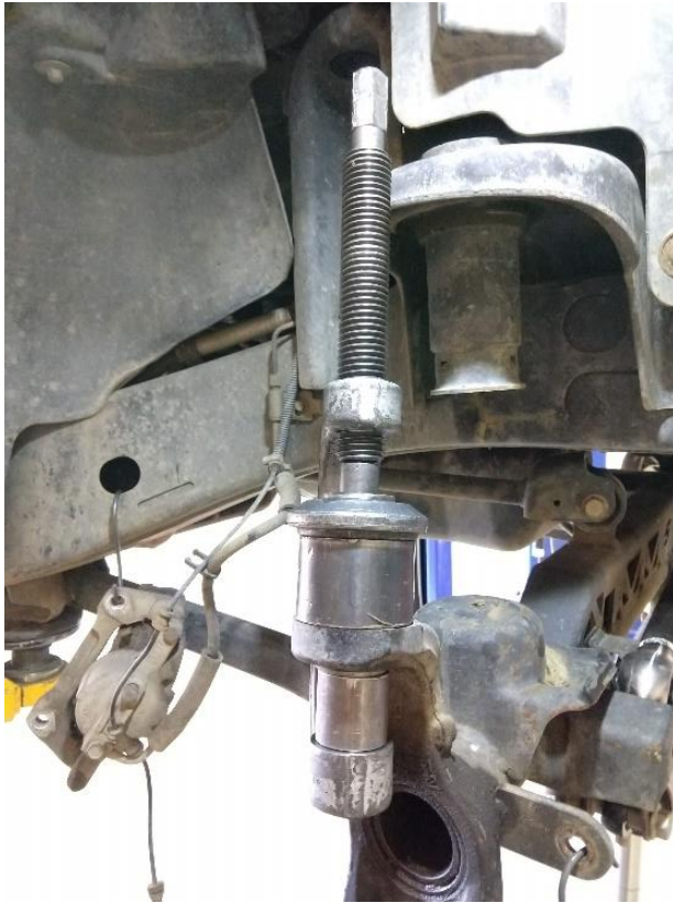
Figure 8. Pressing Out Upper Ball Joint
