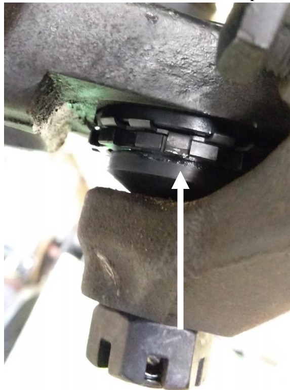
Figure 15. Tab Bent Into Cap
