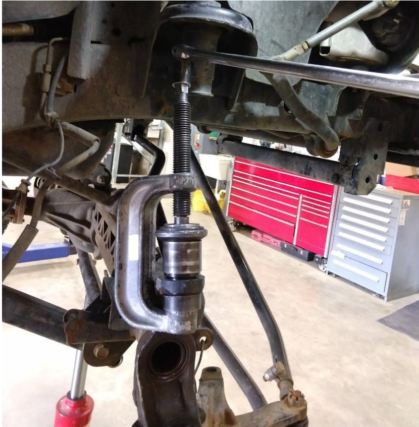
Figure 12. Pressing the Upper Ball Joint into Housing
