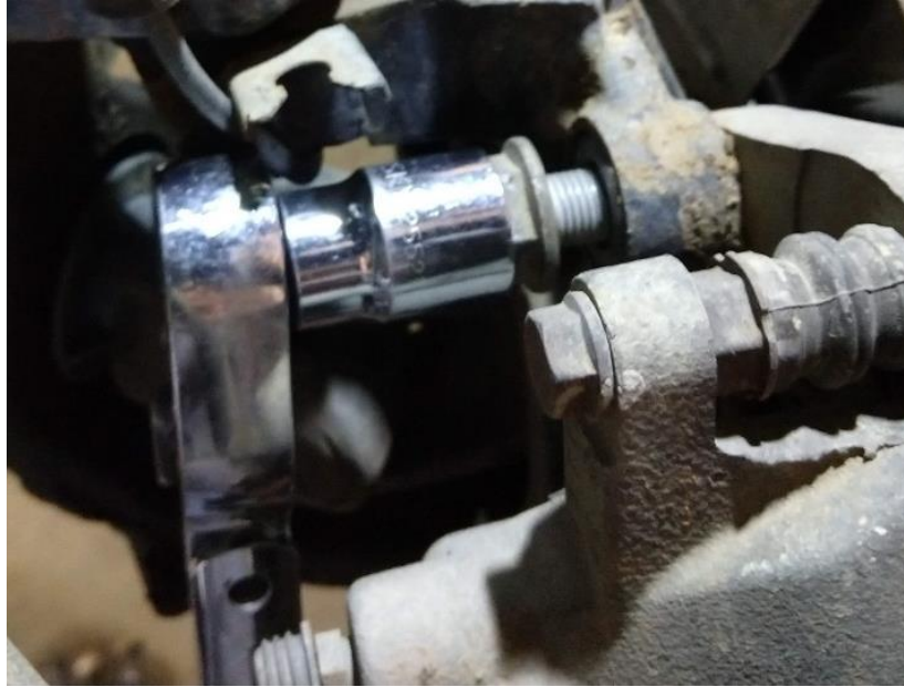
Figure 2. Removing Brake Caliper Carrier Bolts
