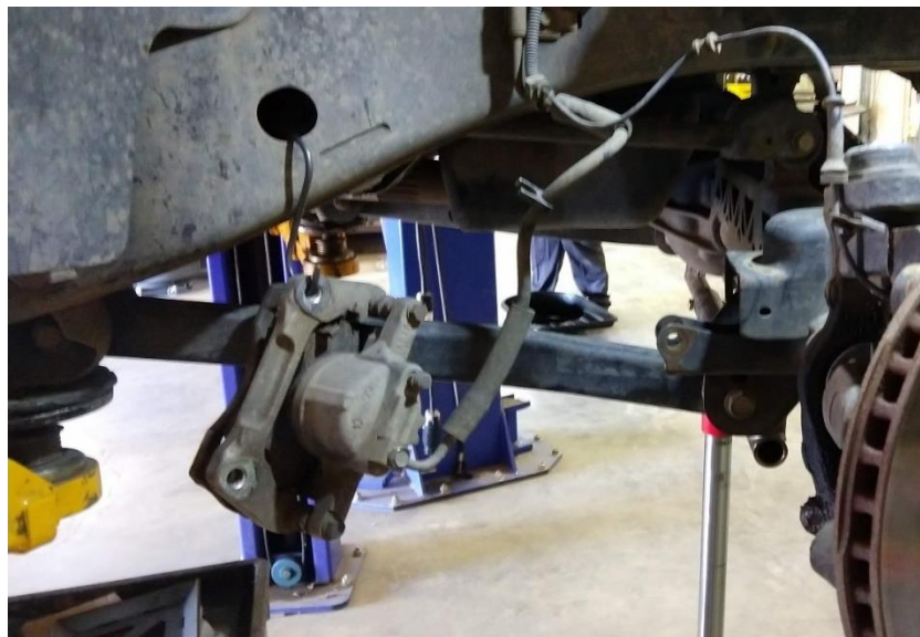
Figure 3. Hanging Brake Caliper
