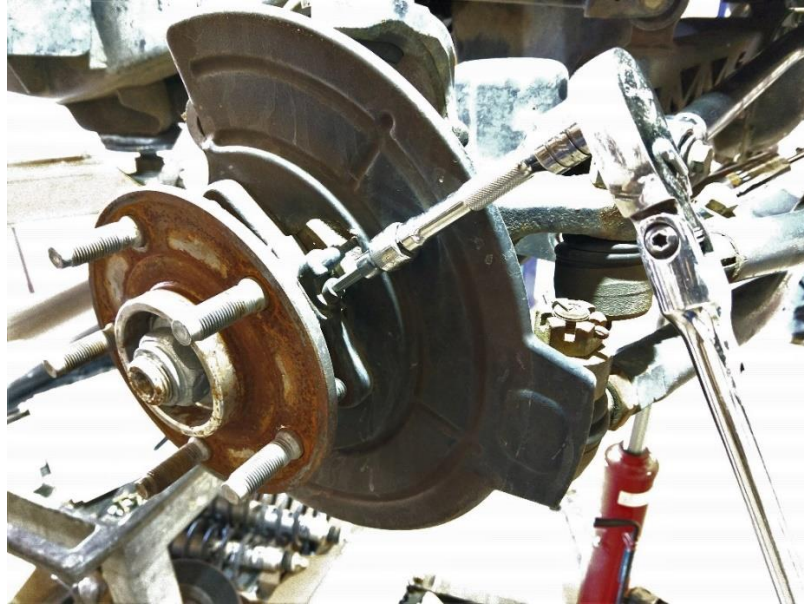
Figure 4. ABS Sensor in Knuckle
