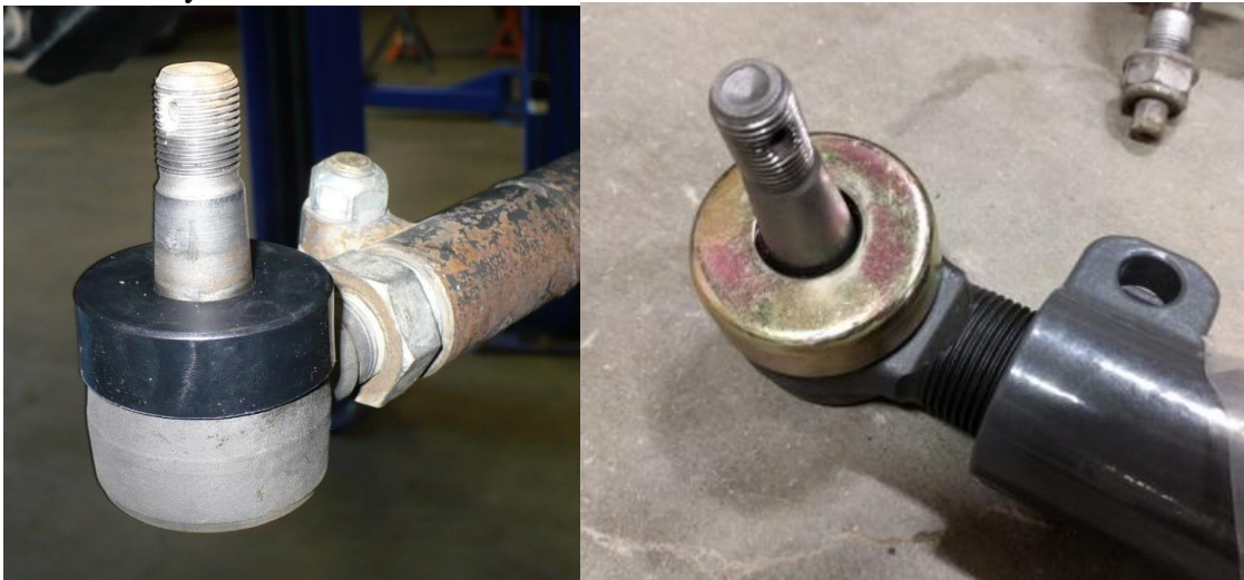
Figures 1 and 2. Dust Boot and Metal Cap Installed On Tie Rod End
