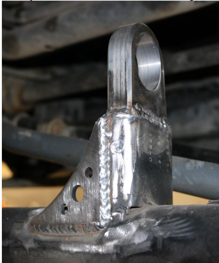
Figure 6. Mount and Gusset Fully Welded
