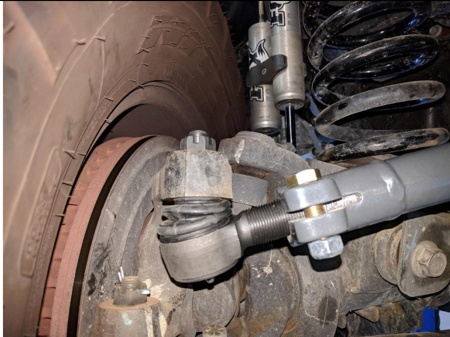
Figure 2. Non-Double Adjuster End of Drag Link at Steering Knuckle
