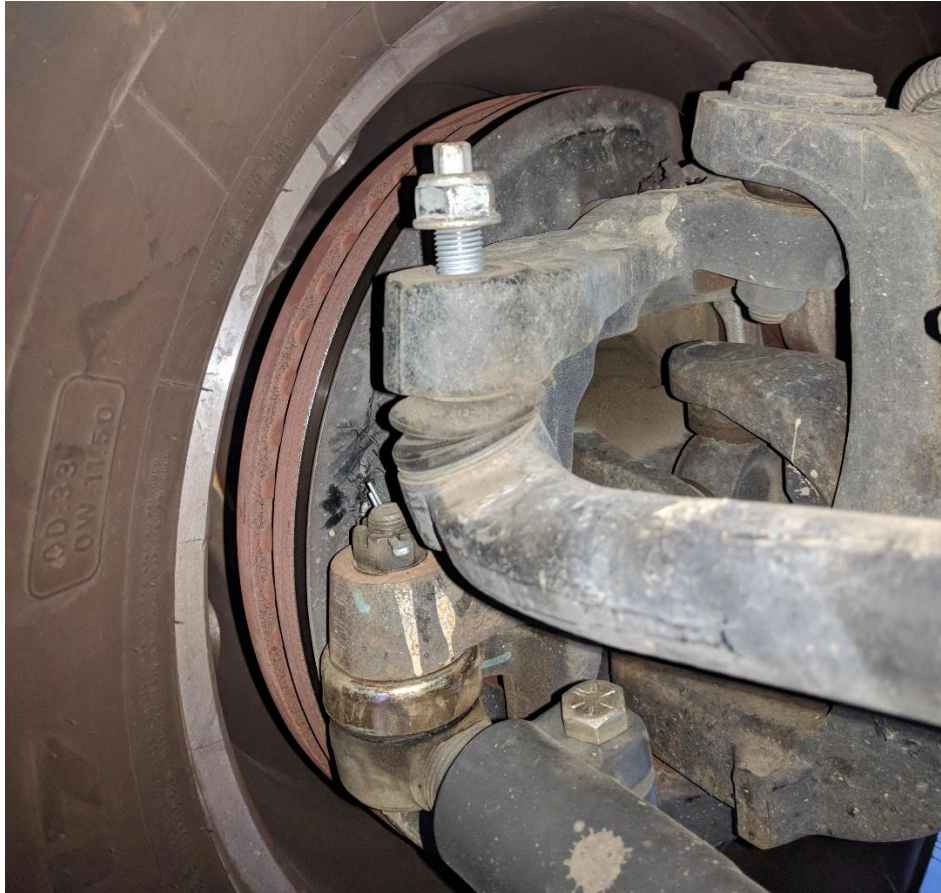
Figure 1. Nylock Nut Loosely Threaded on Factory Drag Link Tie Rod End
