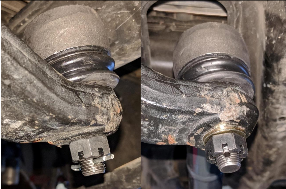
Figure 5 And 6. Washer Used Under Castle Nut in Order for Cotter Pin to Engage Castle Nut
