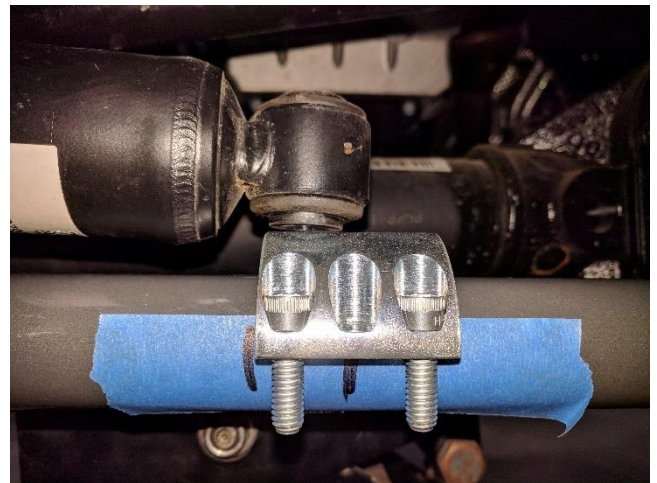
Figure 6. Clamp in Correct Position
