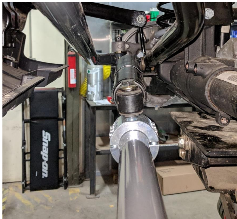
Figure 8. Correctly Oriented Stabilizer and Clamp
