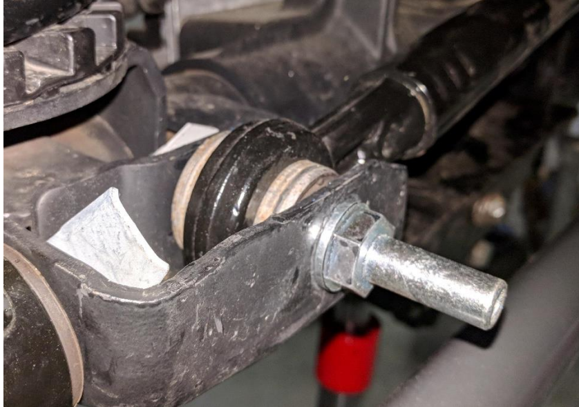
Figure 1. Stabilizer Stud Installed
