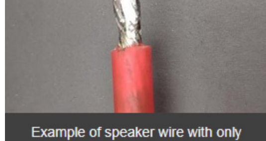
Example of speaker wire with only the tips tinned.
