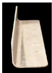
Simple 90° Radius Bend (requires optional radius fingers)
