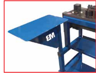
Swing Out Work Tray Holds Follow Bar & Removes for Compound Bends
