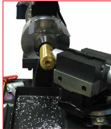
Extended Vise Travel Allows Notching on Either Side of the Cutter
