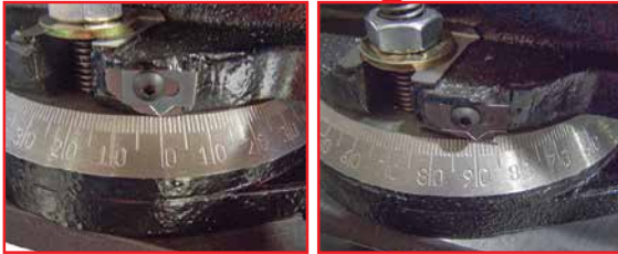
1° Swivel Vise Allows Quick & Accurate Setup!
