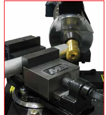
Extended Vise Travel Allows Notching on Either Side of the Cutter
