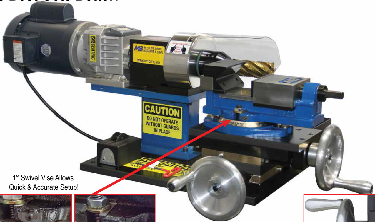
Hand Wheel Calibrated In .013" Segments For Precision Notching
