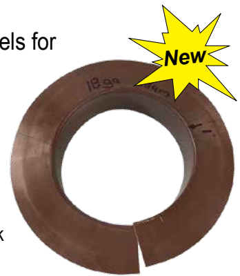
180° Bend Produced Using NEW Stretcher Die # 2700-024
