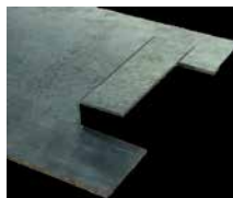
Double Reverse 90° Without Bending Side Legs
