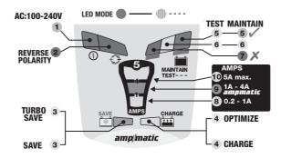
POWER ON: LED #1 - Confirms AC power supply to the charger.
