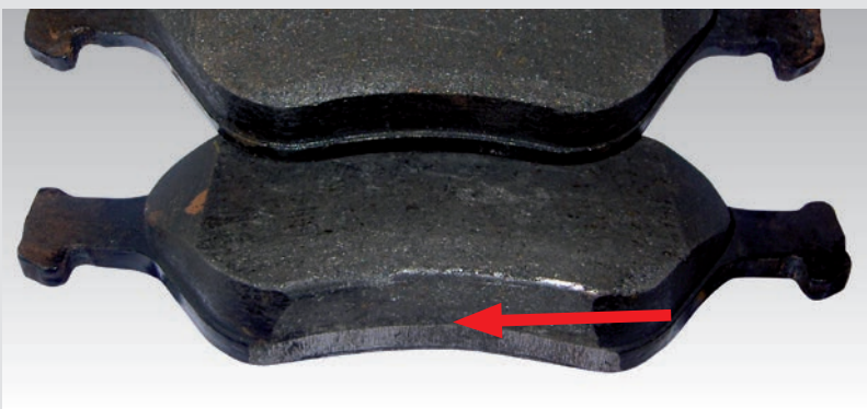
► Improperly changed pad geometry
