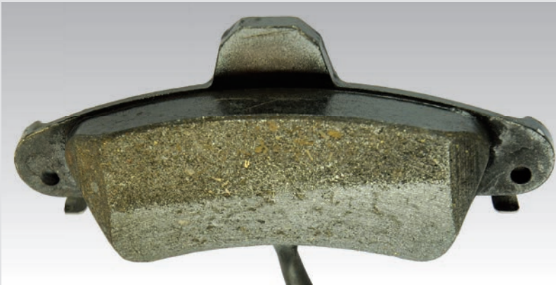
► Pad with inadequate contact pattern
