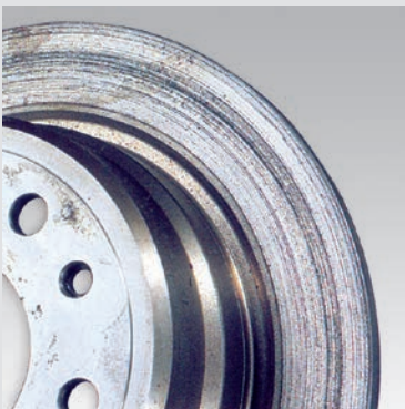
► Brake discs damaged by worn friction material
