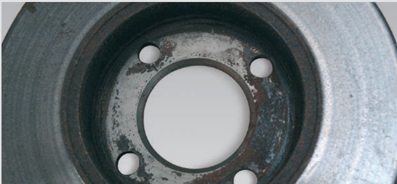
► Heavy underlying corrosion
