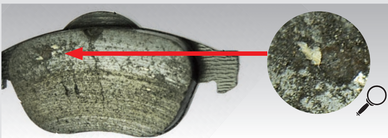
▶ Residues – metal pick-ups in the pad surface
