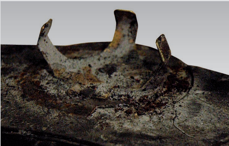
► Cut-out in the damping plate is not functioning due to contamination.
