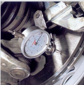
► Measuring disc run-out on the vehicle
