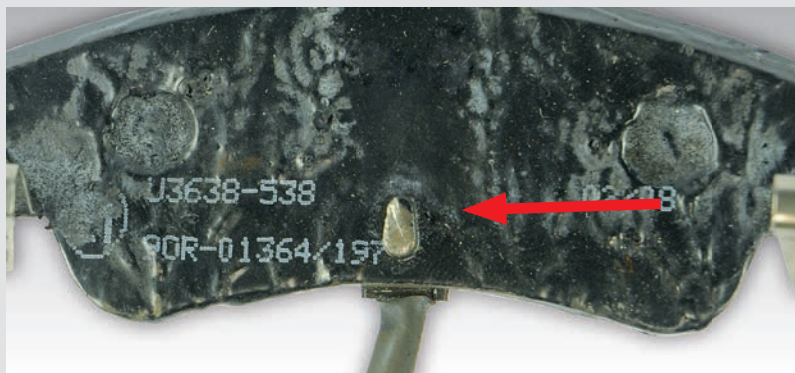
► Piston imprint on the positioning device
