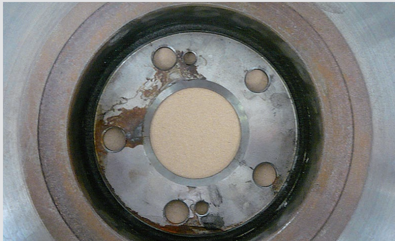
► Cracks in the area of the brake disc chamber
