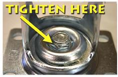
IMPORTANT! After using your creeper for a couple hours (and every month thereafter), please check the tightness of the center swivel nut. After the break-in period the swivel can become loose which will result in the loss of ball bearings. This is not covered under warranty!
