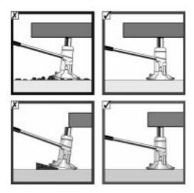
If the load is not centered or the entire face of the plunger saddle does not contact the load, side loading will occur. Side loading creates an unstable setup which may shift or fall. It also damages the jack or cylinder by distorting the wiper seal and bending the plunger. Side loading increases with distance. The further you extend the plunger, the more unstable it becomes.
