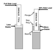
Cylinder Stroke – The illustration at left shows 2 benefits of applying the 80% rule to cylinder stroke. The first is that leaving distance between the stop ring and the bearing reduces side loading force resulting in a more stable cylinder. The second is that you avoid damaging the stop ring by running the plunger all the way up and hitting the stop ring with the bearing.
