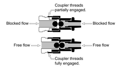
• Couplers are designed to be pressurized only when they are connected together. Never pressurize half couplers.
