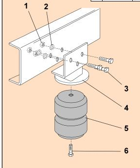
Do not exceed vehicle manufacturer's recommended axle weight rating. Check for AEON® interference with vehicle components - Under load AEON® will "expand" in diameter.
