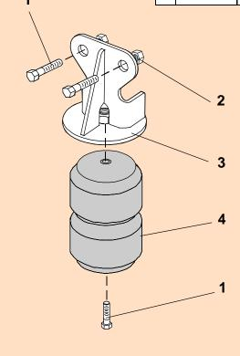
Do not exceed vehicle manufacturer's recommended axle weight rating. Check for AEON® interference with vehicle components - Under load AEON® will "expand" in diameter.
