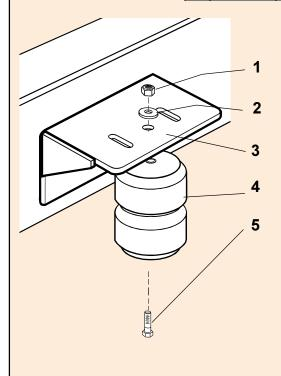
Do not exceed vehicle manufacturer's recommended axle weight rating. Check for AEON® interference with vehicle components - Under load AEON® will "expand" in diameter.
