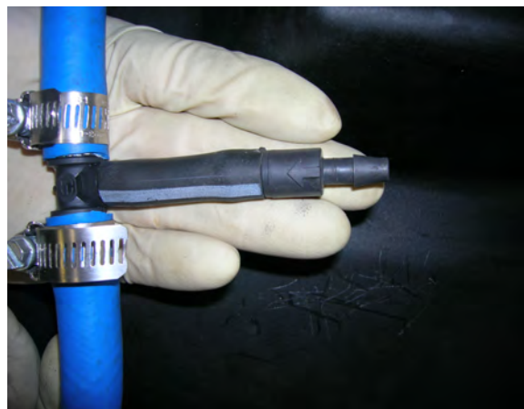
(Fig. 8) The arrow on the \frac{1}{4} " Check Valve MUST point towards the tank vent hose system. When the tank is lifted into the truck the open end of this check valve will be inserted into the end of the existing vent system mounted to the frame of the truck. This prevents vacuum build-up. This is required on all Ford trucks.
