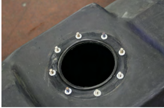
(Fig. 3) Leave the "O" ring gasket, studs and retainers assembled as they are (shown before sending unit, top flange, and 5/16" nylon locking nuts are installed).
