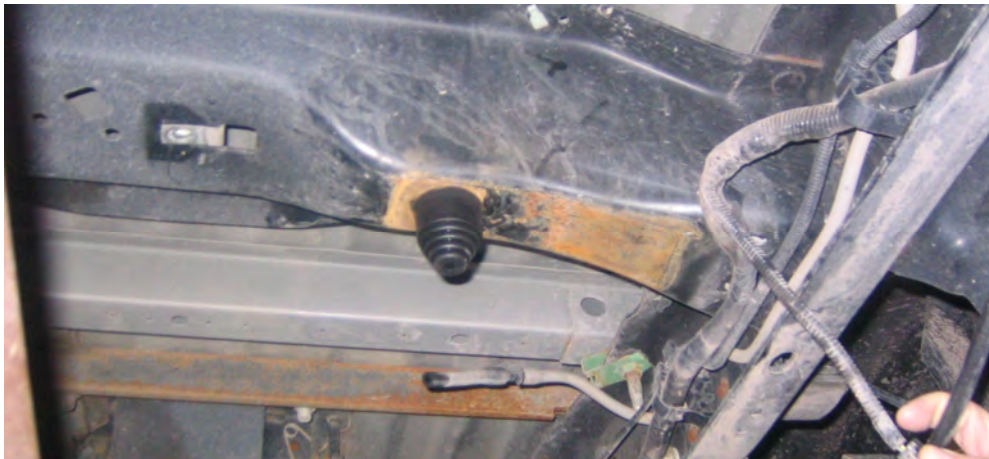
(Fig. S1) The "Fuel Tank Cushion Mount" is shown fastened in place on the cross member.
