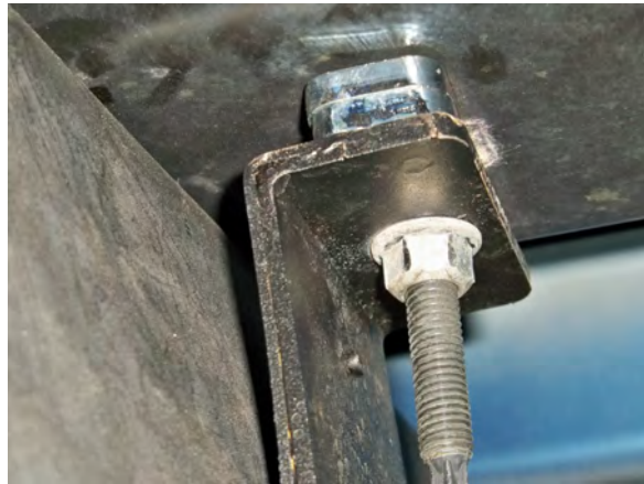
(Fig. 10) Tighten the bolt and bracket against the shims. If the strap does not hold the tank tightly enough, remove one shim at a time until it is tight.
