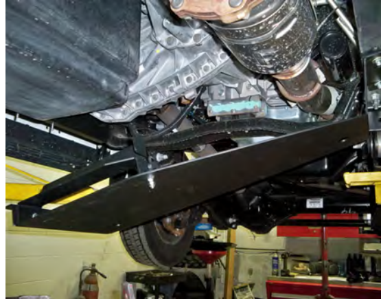
(Fig. 4) Attach the Skid Plate to the bottom of the passenger side of the frame first, leaving the bolts loose. Make sure the Nose Bracket is on the edge of the Skid Plate closest the rear of the vehicle.
