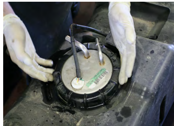
(Fig. 2) Remove the sending unit from the original equipment tank by rotating the hold-down ring counter clockwise.
