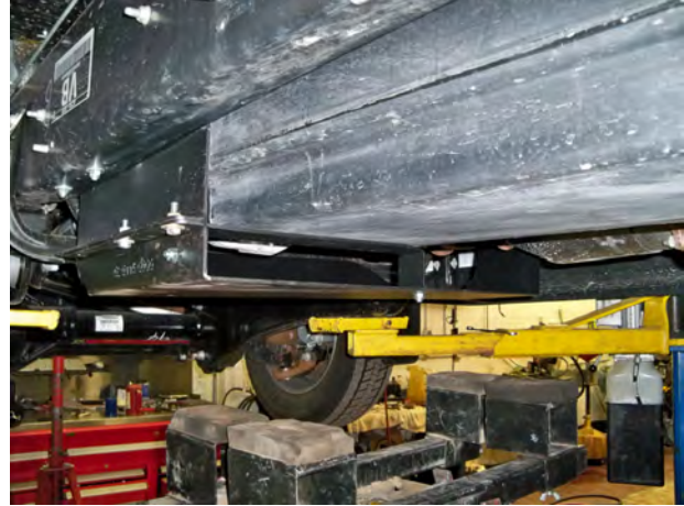
(Fig. 6) Skid plate bolted into place on bottom of formed channel. Note Nose Bracket is in "high" position.
