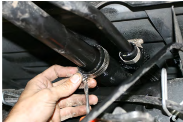
(Fig. 12) Attach fuel tank 1 1/2" fill hose and 3/4" vent hose to vehicle fill spout. Vent hose may have to be shortened about 6 inches to fit properly. On some long bed tanks, 1 1/2" fill hose may have to be extended with 3.35" hose extension.
