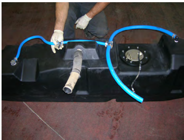
(Fig. 7) LONG BED tank vent hose arrangement. This photo shows how the 90° x \frac{3}{4} " elbow and the front rollover valve are pointed at 45° angles toward each other and the inboard side of the tank. This is different than short bed plumbing. The technician's hand is holding the \frac{1}{2} " x \frac{1}{2} " x \frac{1}{4} " tee with the check valve for the truck's \frac{1}{4} " vent system (See Fig. 8). There is approximately 22" of \frac{1}{2} " hose between the rollover valve and
