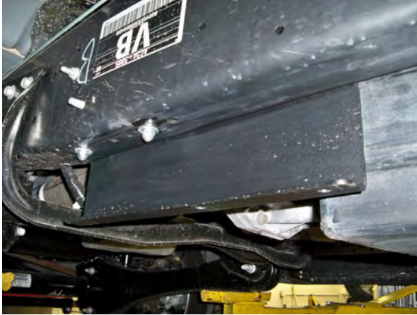
(Fig. 5) Formed channel is bolted to the inside of the frame on the driver's side.
