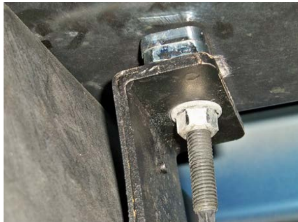
(Fig. 7) Tighten the bolt and bracket against the shims. If the strap does not hold the tank tightly enough, remove one shim at a time until it is tight.
