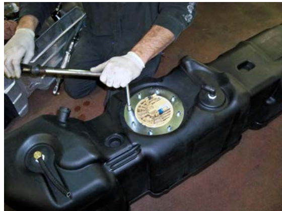
(Fig. 3) Place the sending unit into the TITAN tank, install the top flange, and tighten the nylon lock nuts to 20 ft. lbs using a “star” pattern using a torque wrench.
