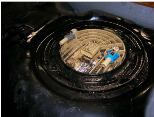
(Fig. 2) Loosen the hold-down ring on the OEM tank by turning counter-clockwise. Note where the connections on your vehicle’s sending unit are “clocked” and install so they are located in the same position in the new tank.
