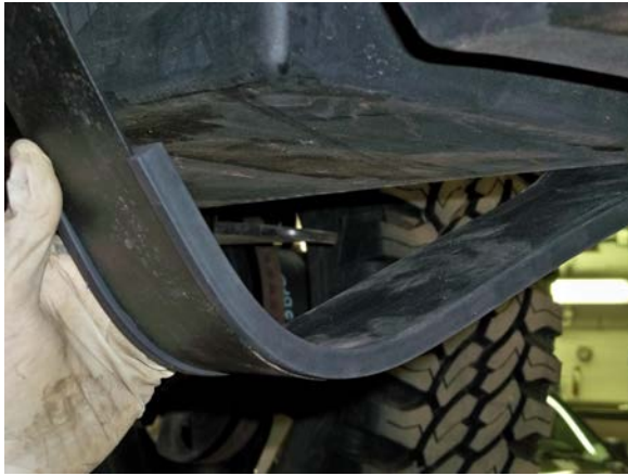
(Fig. 4) If optional TITAN Shield is not to be installed, install rubber bushings (pn 99 0000 0103) on both straps with the channel side toward the strap.
