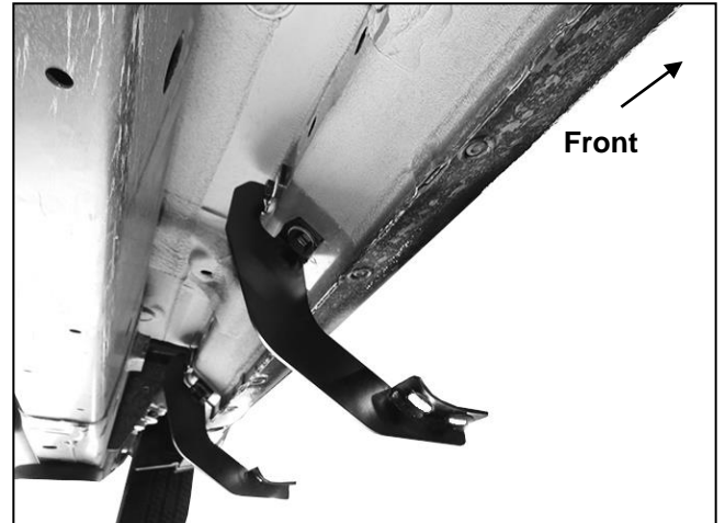
(Fig 6) Driver/Left Center Mounting Bracket installed
