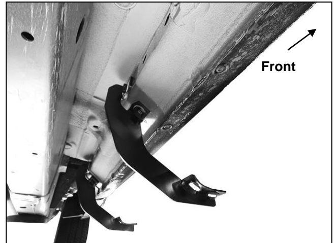
(Fig 6) Driver/Left Center Mounting Bracket installed
