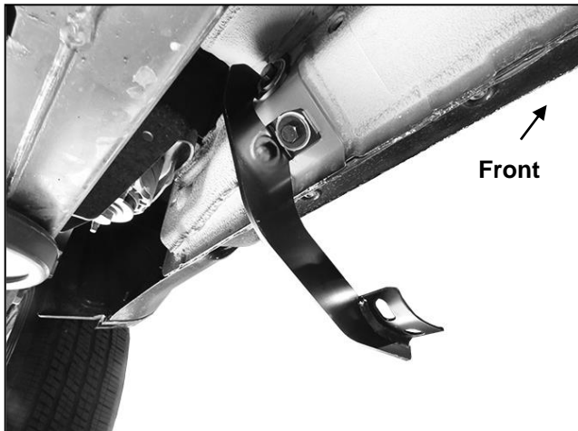
(Fig 7) Driver/Left Rear Mounting Bracket installed
