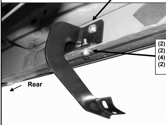
(Fig 3) Driver side-rear Mounting Bracket location
