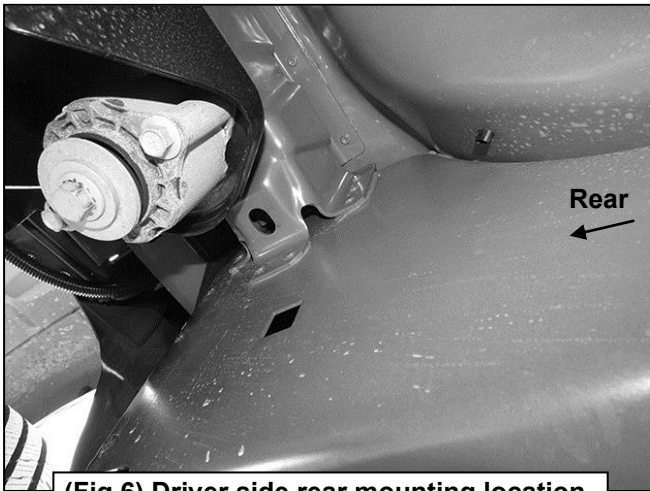
(Fig 6) Driver side rear mounting location
