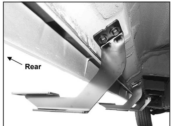
(Figure 7) Attach (2) driver/left #2, #3 and Rear Brackets to the #3 and rear mounting locations.
