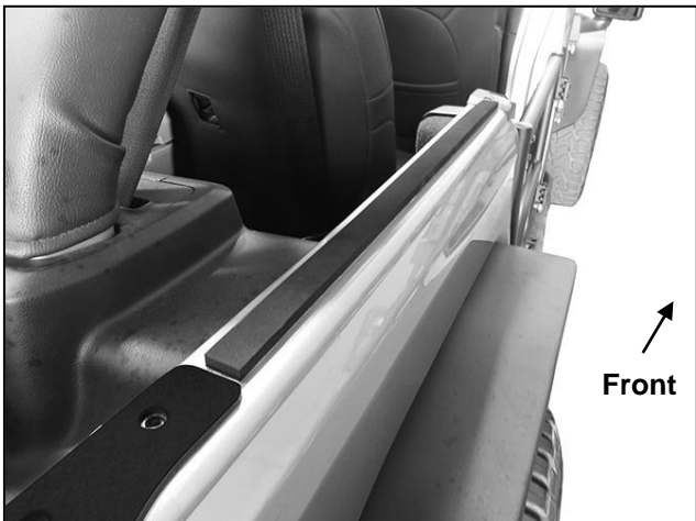
(Fig 16) Install Foam Seal in original location
