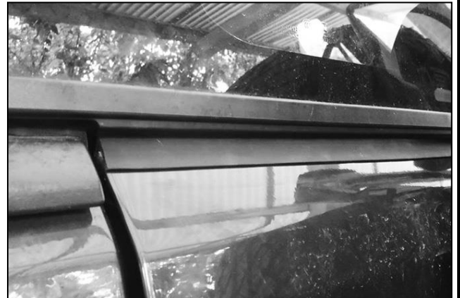
(Fig 26A) Slide Seal over top of tailgate and Tape. Start at end, pull back outer lip on Seal to expose Tape. Slowly remove/pull off outer backing from Tape and stick Seal to Tape and tailgate. Repeat to remove backing from inner Tape on tailgate
