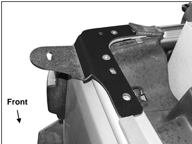
(Fig 14) Passenger/right Mounting Bracket installed
