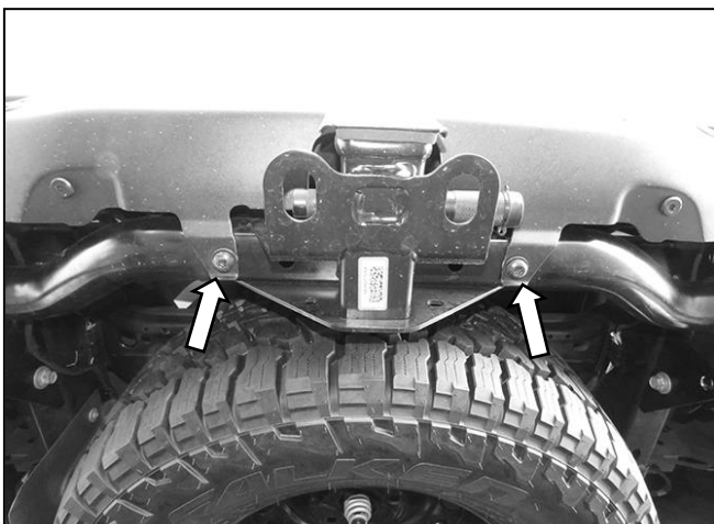
(Fig 3) Remove the (2) bolts under the receiver hitch
