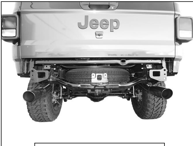
(Fig 8) Factory bumper removed
