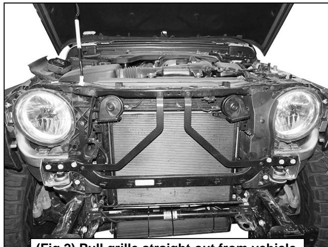
(Fig 2) Pull grille straight out from vehicle to release plastic grille from clips
