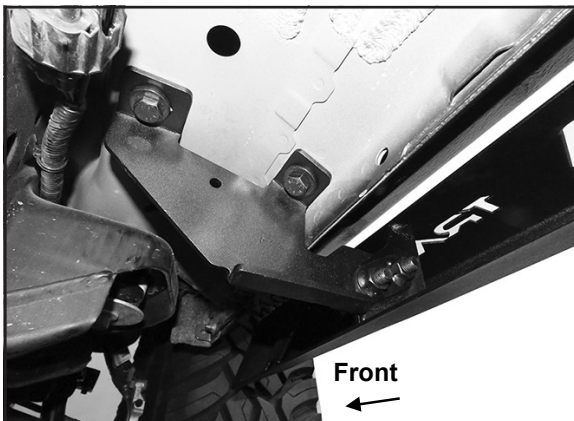
(Figure 11) Passenger/right Side Step attached to Front Mounting Bracket.
