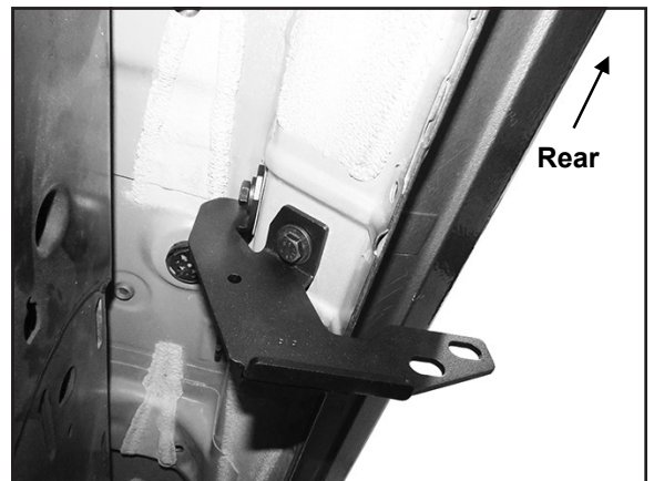
(Figure 9) Passenger/right Rear Bracket installed.
