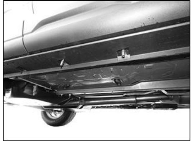
(Fig 13) (2) 10mm Spiral Bolts inserted into the outer center location
