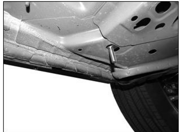
(Fig 9) Insert (1) 10mm Short Bolt Plate into the floor panel
