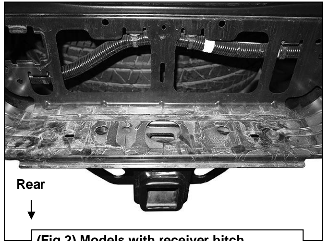
(Fig 2) Models with receiver hitch, remove plastic cover from top of bumper
