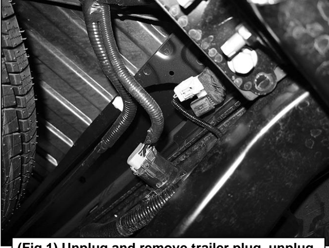
(Fig 1) Unplug and remove trailer plug, unplug license plate lights and sensors if equipped
