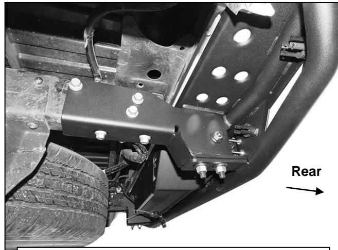
(Fig 12) Bumper attached to Mounting Bracket
