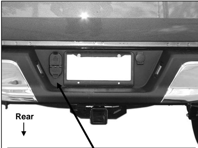
(Fig 1) Unplug and remove 7-wire trailer plug
