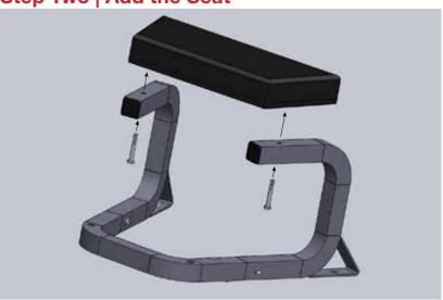
Assemble padded seat onto frame using two bolts.
