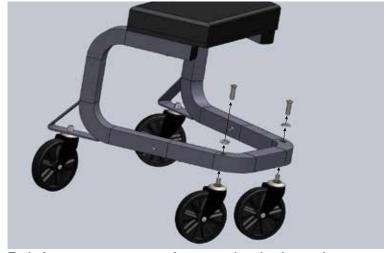
Bolt front casters onto frame using lock washers and barrel nuts.
