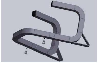
Use set screws to secure frame parts together.
