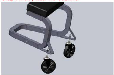
Assemble rear casters using lock washers and nuts.
