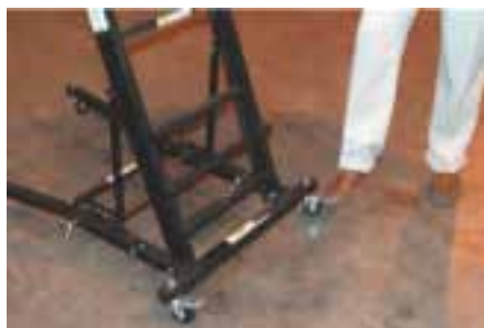
Lock Casters by pressing downward on the locking tab with your foot.
