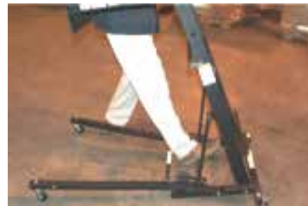
Push the Angle Adjustment Bar forward to the first setting of the notched Angle Adjustment Keeper.
