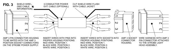
WARNING: All customer supplied wires, that connect to the positive (+) terminal of the battery, must be sized to supply at least 125% of the maximum operating current, and fused "at the battery" to carry the load!
