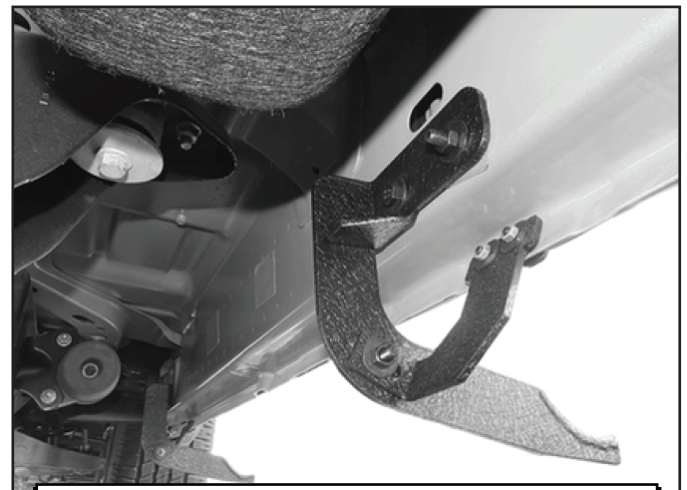
(Fig 15) Passenger/right center Brackets installed
