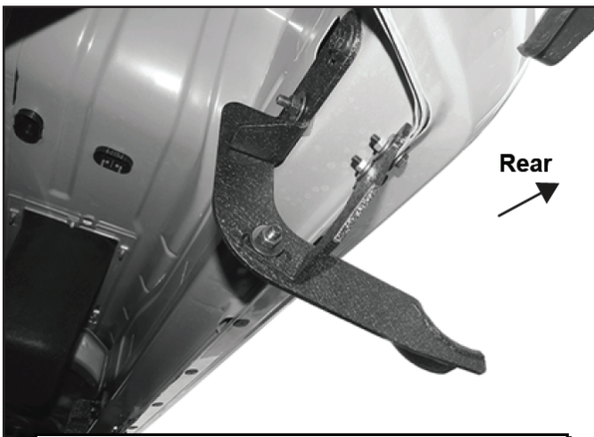
(Fig 17) Passenger/right rear Brackets installed
