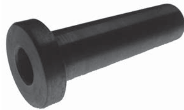
999-3406-225 RIGIDITY BAR MOUNTING BOSS FOR 3/8" BOLT - 5/8" OD x .406" ID x 2.250" LONG
