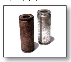
Damaged or improperly installed bushings or sleeves cause uneven movement of the caliper housing.
