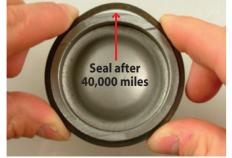
Heat and time dry out the **square-cut seal** and reduce the amount of pull-back as the seal ages. A new seal will pull back the piston about 0.015 inch. In comparison, an old seal may only pull back 0.010 inch or less. If the piston does not retract, it can cause the pads to drag, wearing the pads prematurely.
