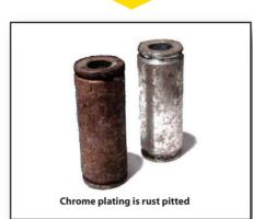
Bushings are pitted and rusted, causing the caliper housing to "freeze" and not move.
