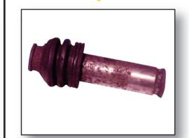
Sliding pins and bushings must be lubed with the proper lube if they are to operate properly.
