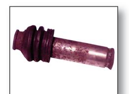
No lubrication on bushings and/or pins prevents free movement.
