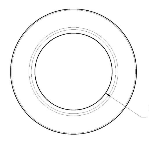
Inside Opening Diameter  $\emptyset_{\overline{16}}^{15}$
