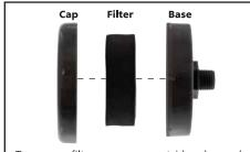
To remove filter cap, grasp outside edge and lift to unsnap. Wash filter with mild detergent and warm water. Rinse and air dry completely before using. Carefully reassemble making sure that filter is setting in the proper location on the base.
