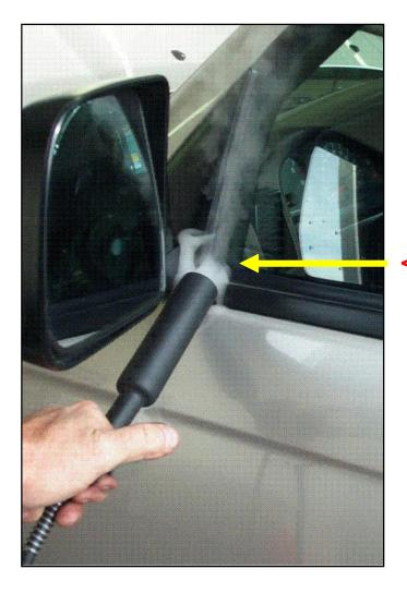
Smoke distrubance pinpoints the leak
