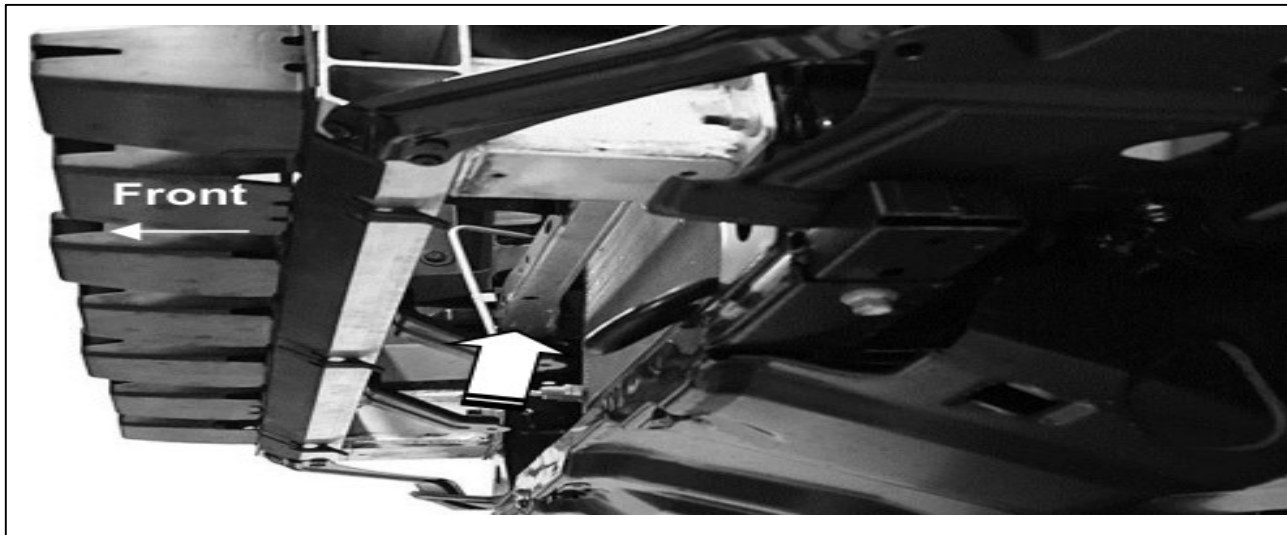
Fig4: Plastic bumper removed for instruction purposes only-do not remove bumper, Locate the outer holes in the bottom of the radiator cross support (arrow) viewed from below.
