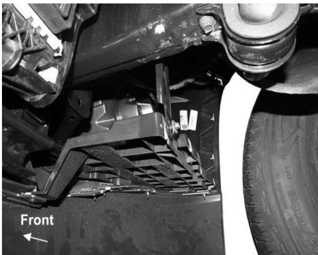
Fig4D: Pull back fender liner to access Bumper hardware and unplug light if equipped
