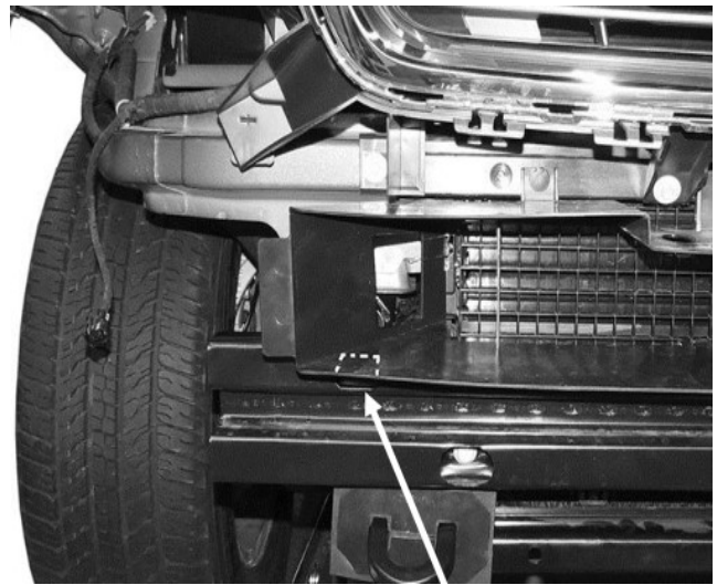
Fig8: Air deflector cut to clear Top Bracket (NOTE: Grille Guard installed to align Top Brackets before tightening 10mm x 80mm Hex Bolts)
