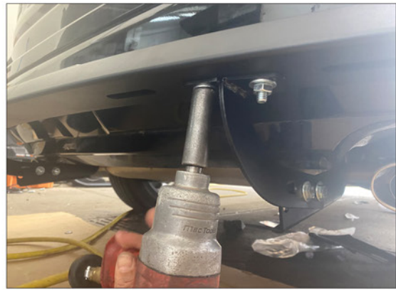
7.Reinforce the bumper with an air gun and wrench.
