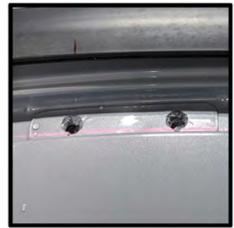
The mounting holes are covered by adhesive stickers in the front middle and rear of the vehicle
