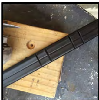
For the alternate trimming technique use an angle grinder or rotary tool to cut through
