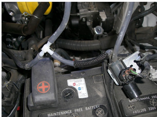
T-FITTING HOSES CONNECTED
